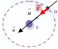
$$\begin{aligned} \sum \vec{F}_{ext} &= m \cdot \vec{a}_G \\ \vec{F}_{E/D} &= m_D \cdot \vec{a} \\ -\frac{GM_E \cdot m_D}{r_D^2} \vec{u} &= m_D \cdot \vec{a} \Rightarrow \vec{a} = -\frac{GM_E}{r_D^2} \vec{u} \end{aligned}$$
